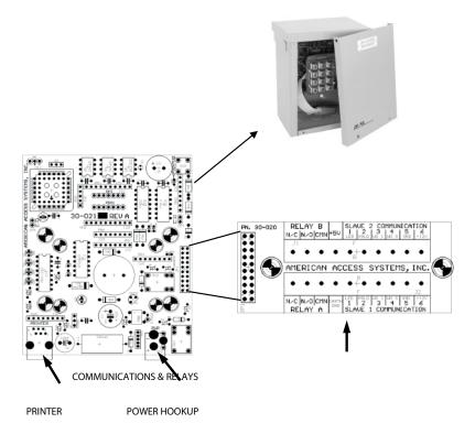
(A). Make all your prox slave connections BEFORE you apply power to the master unit. To connect power to your new desk unit plug the wall transformer into an outlet and insert the other end in the back of the unit.
