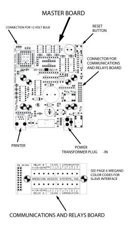
(A). Make all your prox slave connections BEFORE you apply power to the master unit. To connect power to your new desk unit plug the wall tranformer into an outlet and insert the other end in the back of the unit.
