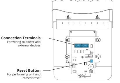
Unit shown with front panel fully open. Internal wiring not shown for clarity.
