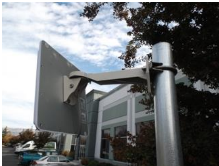
Figure 3. LR-MB with LR-3000 reader, clamped to round pole.
