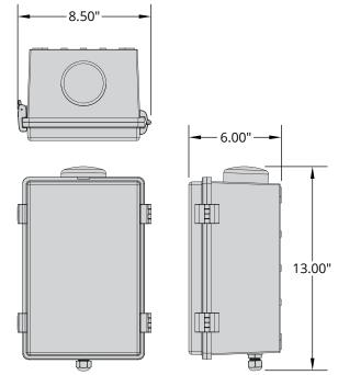
Unit includes one (1) pre-installed 3/8" NPT cable gland for wiring.
